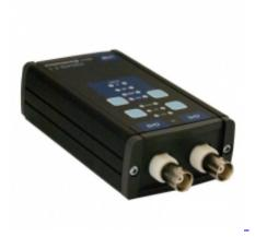
VIBdaq 2.1 is a double channel data acquisition module for signal processing in IEPE standard. Device's inputs can be also configured as AC or DC inputs. The selected input type is indicated by an appropriate diode on the panel, and can be switched using proper buttons. The device is fully powered from USB port. The small size and weight make the device very convenient to use.
